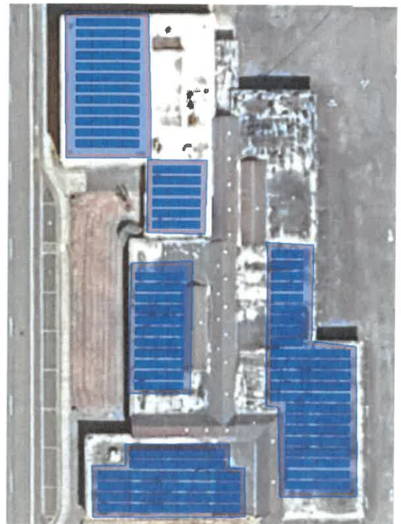
Figure C 125 kW Solar rooftop design
